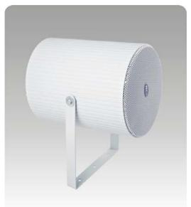
The built-in two 6" full range speaker drivers are designed of wide frequency response 110-15kHz, the multiple power taps 5W, 10W & 20W are helpful for different applications varies from room size and ambient noise surroundings.
