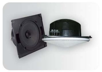
The built-in 6.5" speaker driver is designed of wide frequency response 150-15kHz, the multiple power taps 3W & 6W are helpful for different applications varies from room size and ambient noise surroundings. The metal grille and ABS baffle are painted in attractive RAL9016 white color and a ABS back cover is supplied. Its spring clamp makes the easy and secure installation.
